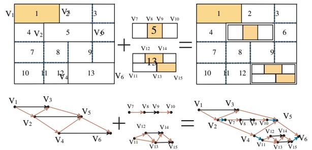
Fig. 4. The Dependency graph for a multi-level treemap.
