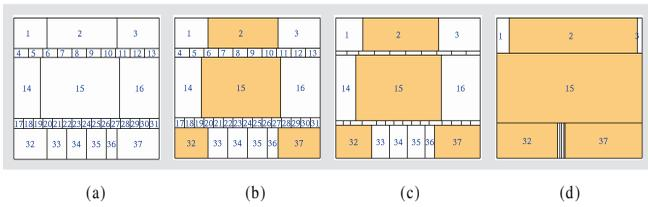
Fig. 1. Desired effects of the seamless focus+context technique on treemaps. (a) the original treemap. (b) foci are selected and colored. (c) foci are enlarged slightly. (d) the state when the foci are maximized.
