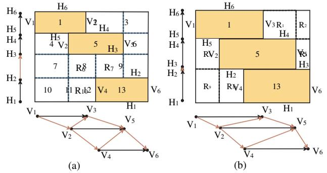
Fig. 3. Dependency graph example: (a) shows the dependency graph for both dimensions in  $TM_{original}$ . (b) shows that the positional dependencies are preserved in  $TM_{transformed}$ . The graph on the left side of a treemap is for the dependency of horizontal edges, and the bottom graph is for the dependency of vertical edges. Different colors are used to distinguish the edges introduced by a focus or non-focus enclosure.
